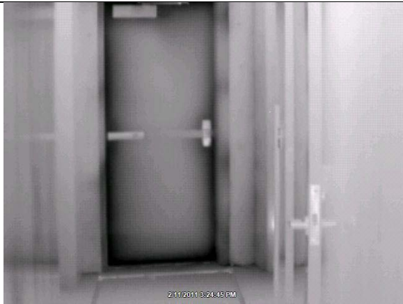
Figure 11 another door showing air leakage at the perimeter.
