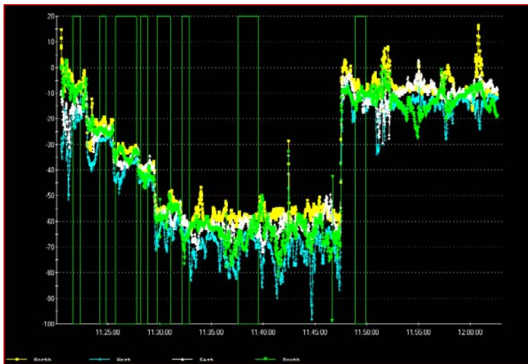
Figure 4. Screen-shot of depressurization test. Colored lines represent the indoor/outdoor pressures. The green rectangles represent periods of records i.e. data used for analysis.
